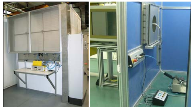
Mixing chamber with air intake filter and aerosol generation (droplet aerosols and dust); right: interior view
