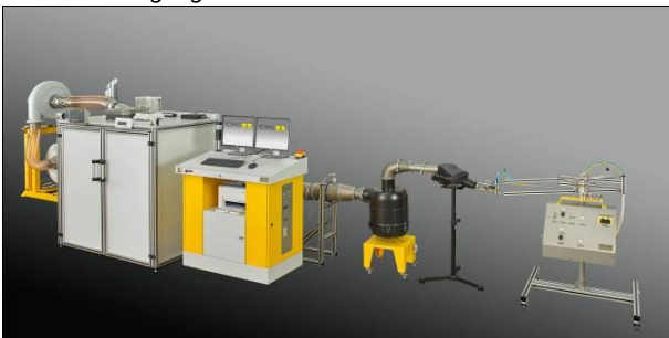
Test Rig ABP 115 with water injection system and water separator
