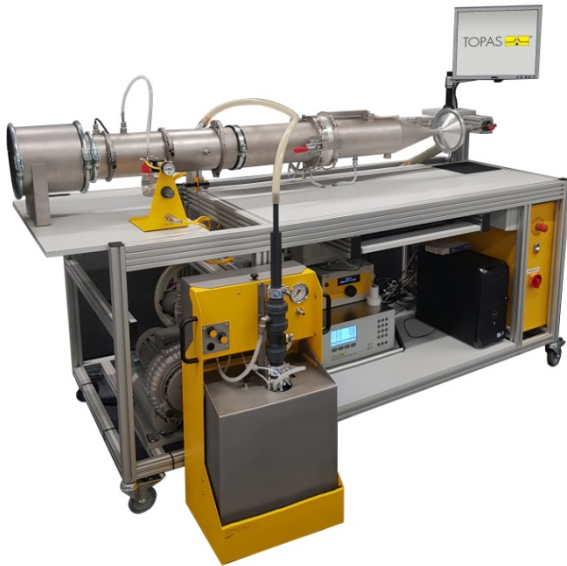
AFC 132 Filter media test rig according to ISO 16890
