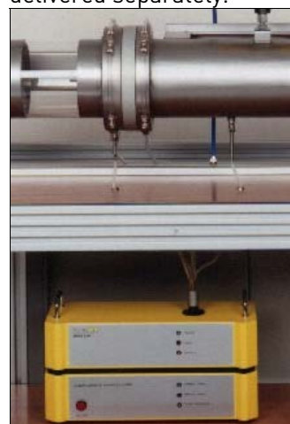
Effective measurement of particle size distributions with a laser aerosol particle size spectrometer LAP 322 (arrangement with sample switching unit below the test channel)
