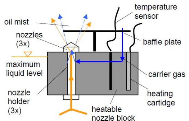
Schematic of the nozzle assembly
