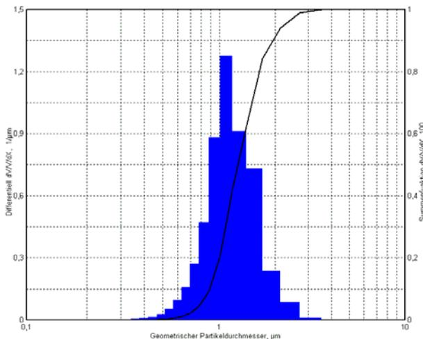
Particle size distribution of an aerosol generated by the ATM 243 with a  $d_{50} < 1.5 \mu\text{m}$  (Motor oil 15W40, 130°C)
