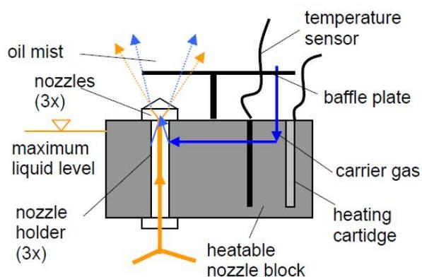
Schematic of the nozzle assembly
