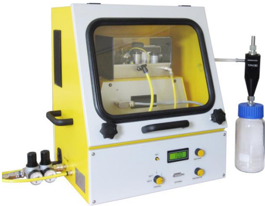
Dust Generator Unit (DGU 413) with SAG 410/U and cyclone.
