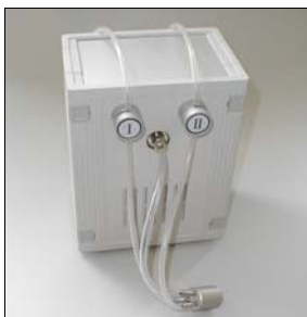
SYS 520 with adapter for particle measuring device
