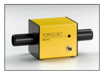
Process Aerosol Photometer PAP 612 with connection cable for power supply and data transfer
