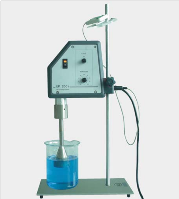
Device for supporting microsieving process: ultrasonic disintegrator UDS 751/UP 200S
