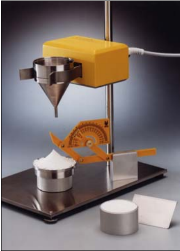
Determination of angle of repose with EMS 755
