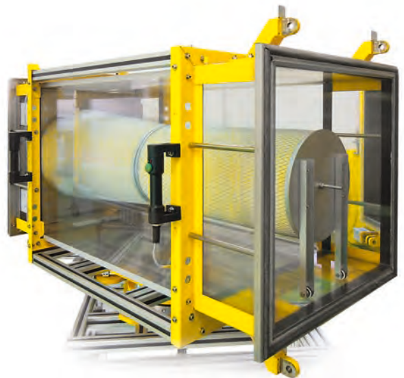
盒状过滤器的夹具 Cartridge Filter Holder
